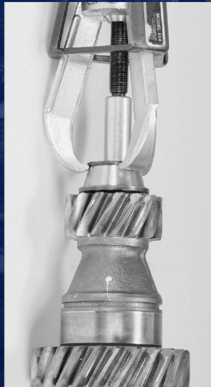
Clamps an failed bearing surfaces
