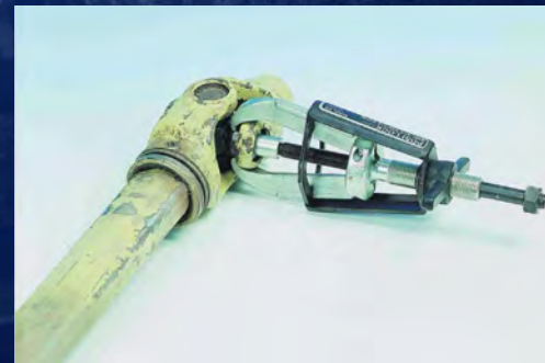
U-joint removal and installation
