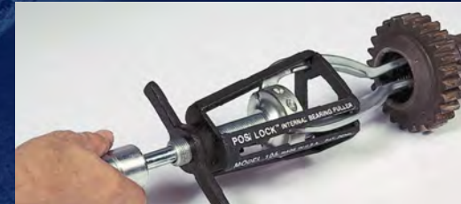
Needle bearing removal from transmission gear
