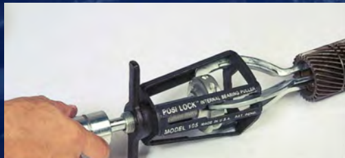
Bushing removal from transmission gear
