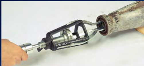
Oil seal removal from transmission housing
