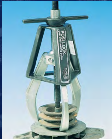
Alternator pulley removal
