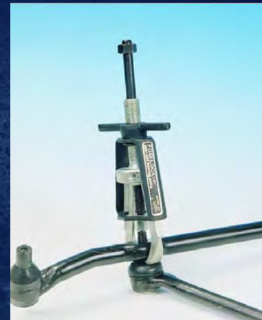
Steering linkage removal
