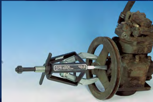
Hydraulic pump pulley removal (Model 106)
