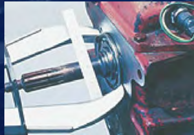
Jaws fit in snap ring grooves as narrow as .070in (1.78cm)
