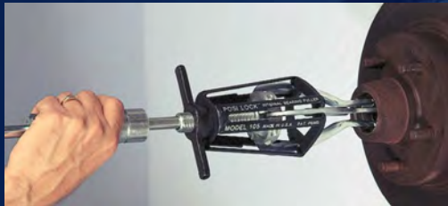
Bearing cup removal from brake rotor
