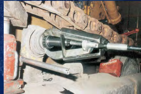
Dozer's bearing removal (Model 116)
