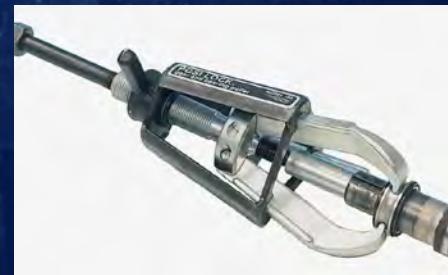
Removal of bearing races
