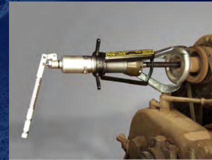
Removal of a hand wheel from a lathe
