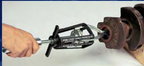
Pilot bearing removal from crankshaft
