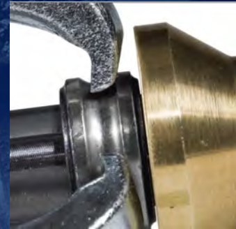
Locks on ball grooves and bearing races
