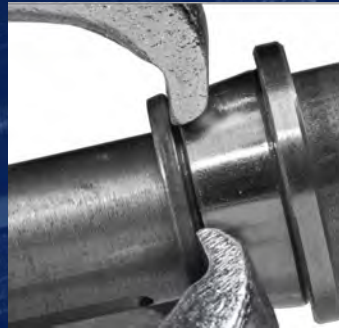
Remove tapered roller bearings
