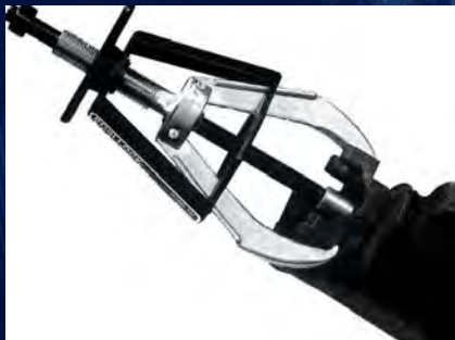
Transmission and rear end yoke removal
